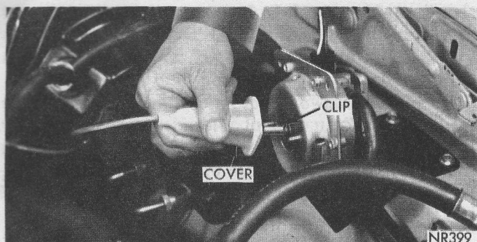
Fig. 13—Removing/Installing Throttle Cable Cover
